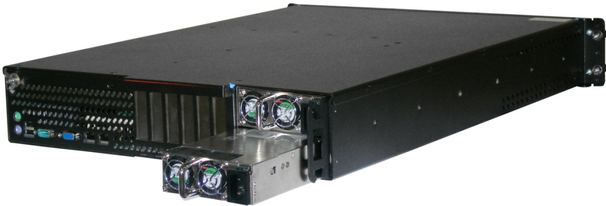
Figure 6-21 Hot-Swap of 2U Server Power Supply Module
